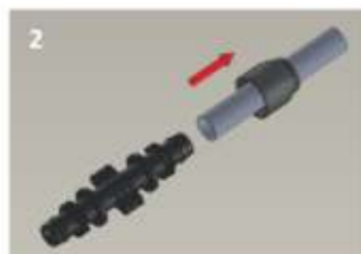
Pull the coupling nut up to the end of the pipe
