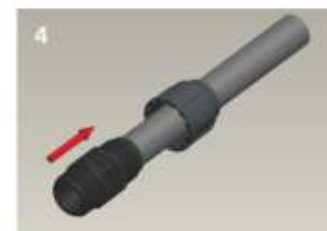
Insert threaded part of body on the free side of the grip ring
