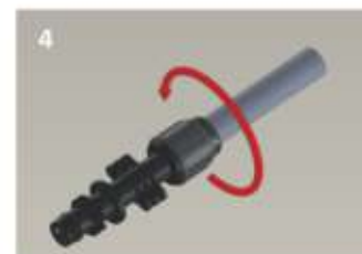
Pull back the nut and coil it completely on the fitting
